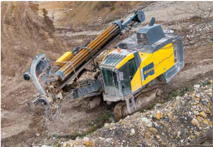
To access the limestone seam, Buffalo Valley Resources uses its Epiroc FlexiROC D65 surface drill rig to drill precise blast holes before shooting the material.
