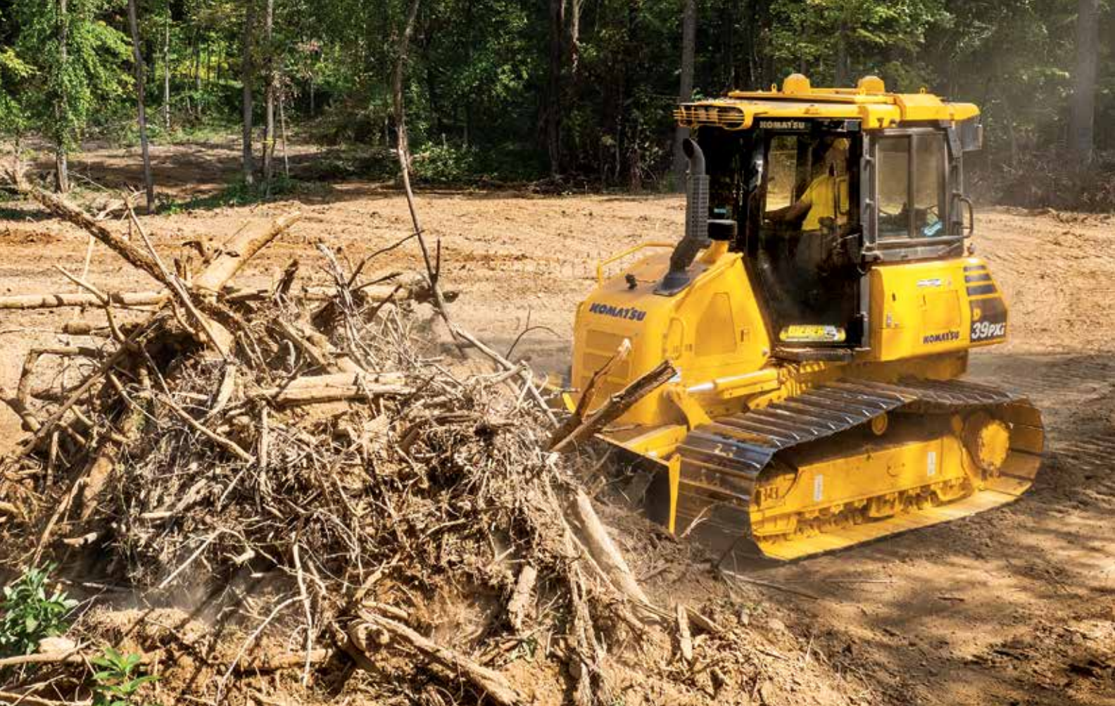
With a Komatsu D39PXi-24 Intelligent Machine Control (IMC) 2.0 dozer, an operator moves material without going below grade.
