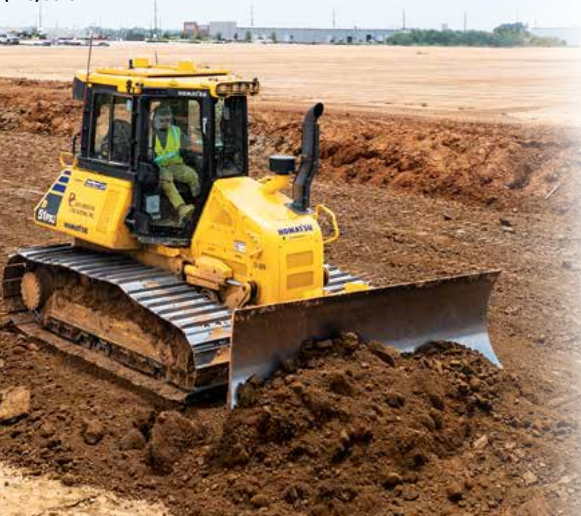
An operator cuts to grade with a Komatsu D51PXi-24 Intelligent Machine Control (IMC) dozer.
