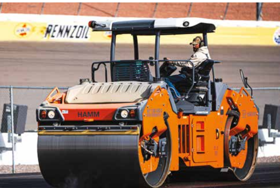
HAMM's HD+ 120i VIO-2 HF offers versatility with two VIO drums that enable a total of nine different compaction mode combinations.
