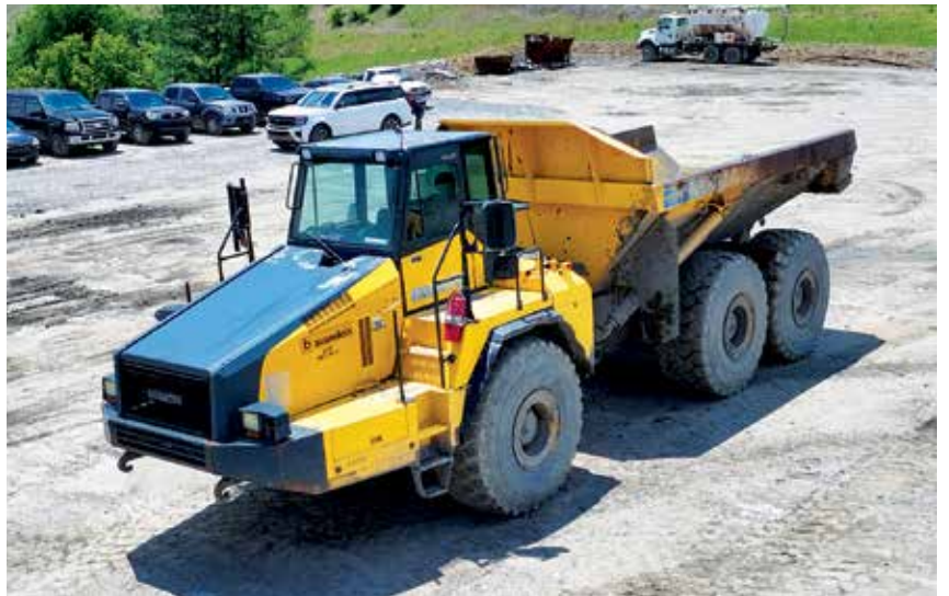
To move material around its mining operation, Jigsaw utilizes Komatsu HM400 articulated trucks.
