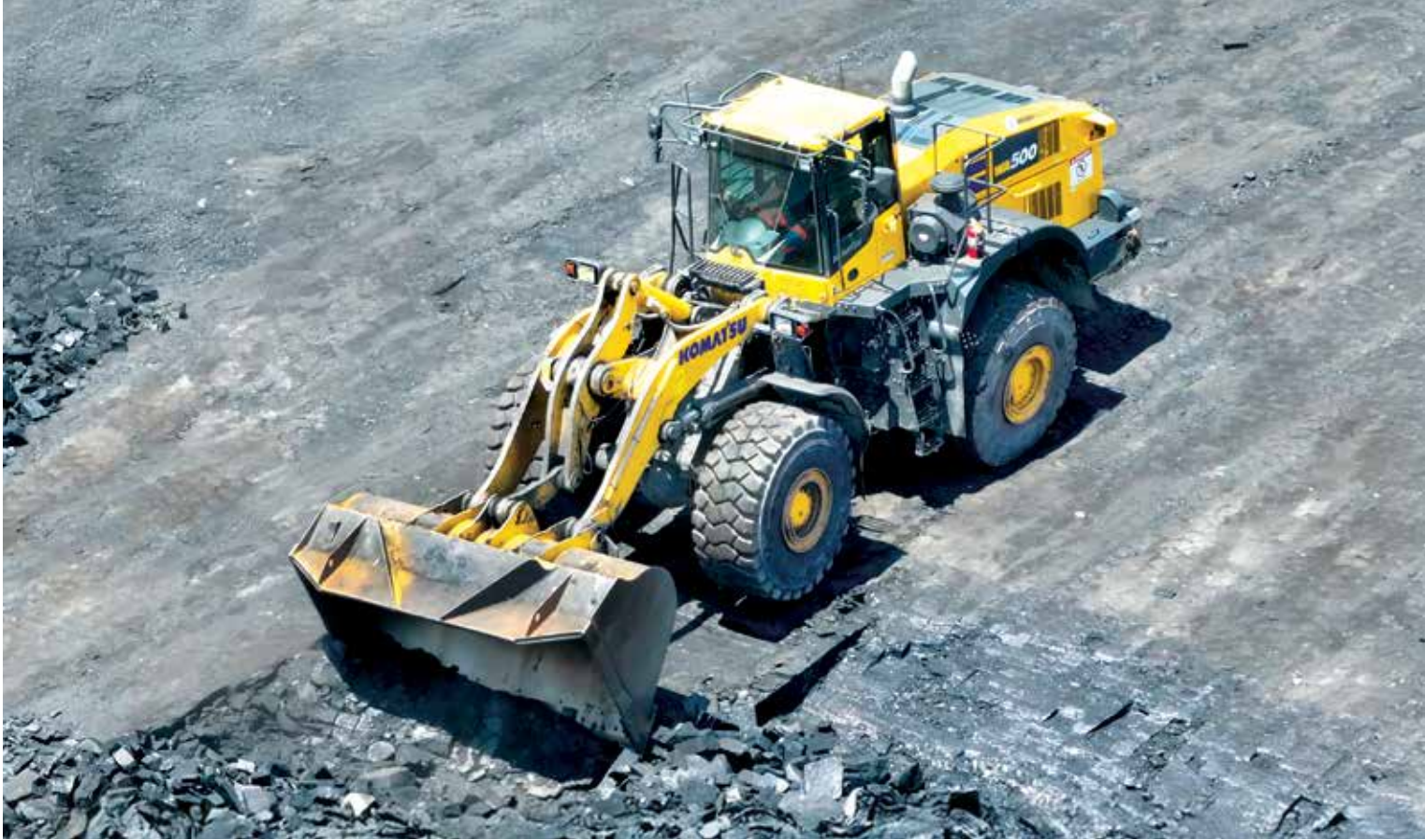
An operator pushes a pile of coal with a Komatsu WA500 wheel loader.
