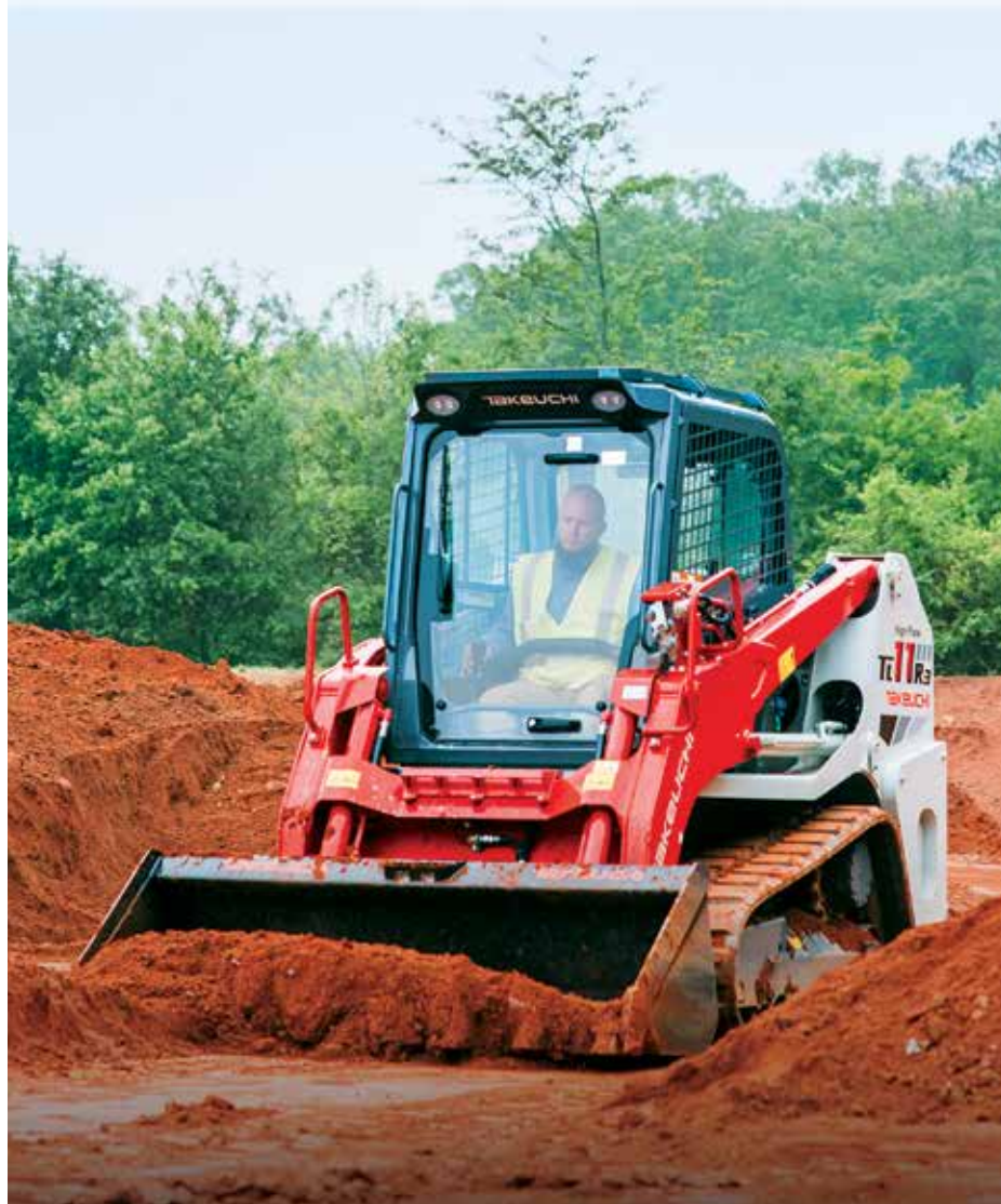
Takeuchi's TL11R3 compact track loader features new electric-over-hydraulic (EH) controls for greater precision in loader arm, bucket and travel speed operation.
