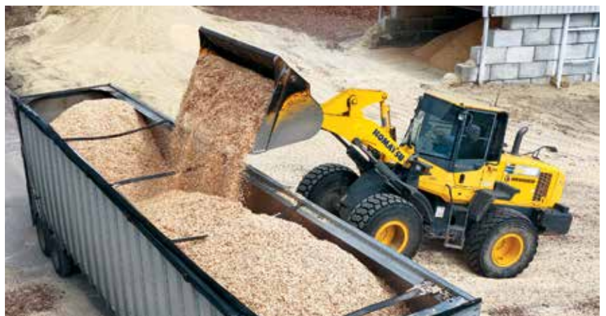
Swapping out forks for a bucket on the Komatsu WA200 wheel loader allows operators to easily load semi-trailers with chipped material to be shipped to the surrounding region.
